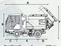
Overall Length Overall Height Front Overhang Rear Overhang Wheelbase Tipping Height Overall Width **Turning Circle**
