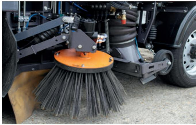
Trailed, robust, steel suction nozzle for durability. Complete with trailed side brush, widesweep brush and optional front brush assemblies all fitted with water nozzles for dust suppression.
